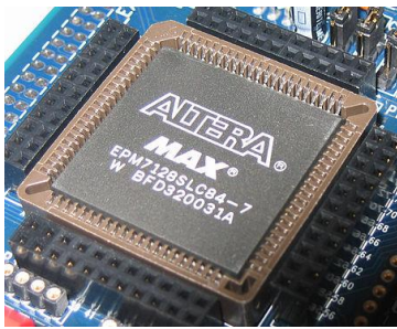
An Altera MAX 7000-series CPLD with 2500 gates.
