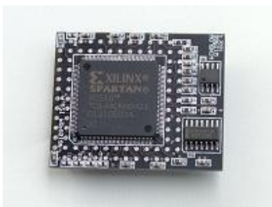
Original Adapter design (2002) utilised Xilinx XCS10-3TQ144C & XC17S10V08C. Last time buy announced 2010
