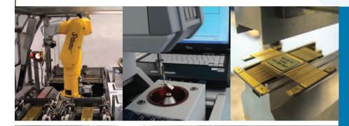
The MicrossSXT automated solder-dipping process mitigates tin-whisker formation to increase component reliability.
