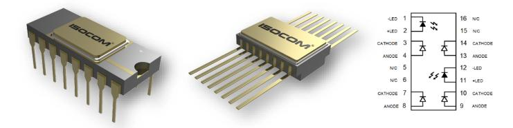
The CDL400 and the CDSML400 are hermetically sealed linear optocoupler devices, consisting of an LED optically coupled with two photodiode detectors. Package styles for these devices include a 16-Pin DIP package for the CDL400 and a 16-Pin flatpack package for the CDSML400 with lead form options and solder dip options available.
