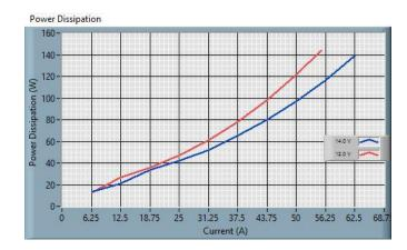
Fig. 4: 48S12.3K0BCA Power Dissipation - Boost Mode Vo=48V
