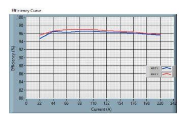
Fig. 1: 48S12.3K0BCA Efficiency Curve - Buck Mode, Vo=14V.
