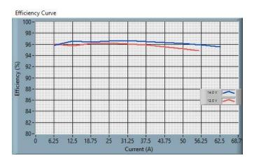
Fig. 3: 48S12.3K0BCA Efficiency Curve - Boost Mode, Vo=48V
