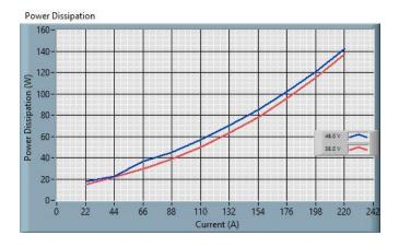
Fig. 2: 48S12.3K0BCA Power Dissipation - Buck Mode, Vo=14V.
