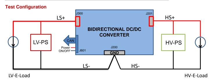
Fig. 2: The bench setup used to operate 48S12.3K0BCA and take measurements provided in data sheet. The combination of the Electronic Load (E-Load) and Bench Power Supply (PS) emulates a battery capable of both sourcing and sinking current.
