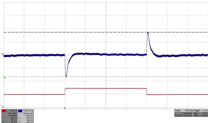
Fig. 53: Output voltage response to load current step change 50% - 75%-50% (9.5A-14.25A-9.5A) with di/dt = 1A/\mu s at V_{in} = 24V . Top trace (C4): Output voltage (200 mV/div.). Bottom trace (C3): Load current (10A/div.). Time: 1ms/div.
