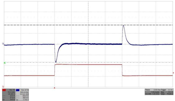
Fig. 48: Output voltage response to load current step change 50% - 100%-50% (10.5A-21A-10.5A) with di/dt = 1A/\mu s at V_{in} = 24V . Top trace (C4): Output voltage (500 mV/div.). Bottom trace (C3): Load current (10A/div.). Time: 1ms/div.
