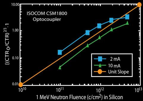
Fig. 4. Values of  $[(CTR_0/CTR)^{1/3} - 1]$  for  $I_F = 2$  and 10 mA for CSM1800.
