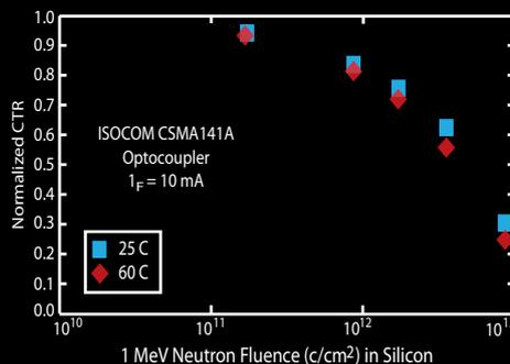
Fig. 7. Normalized CTR versus the radiation level for room temperature and 60°C for CSM141A.
