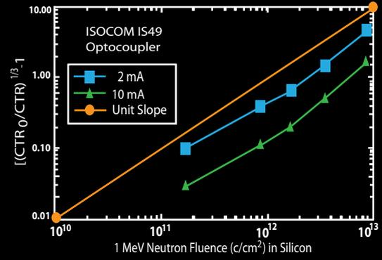
Fig. 2. Values of  $[(CTR_0/CTR)^{1/3} - 1]$  for  $I_F = 2$  and 10 mA for IS49.
