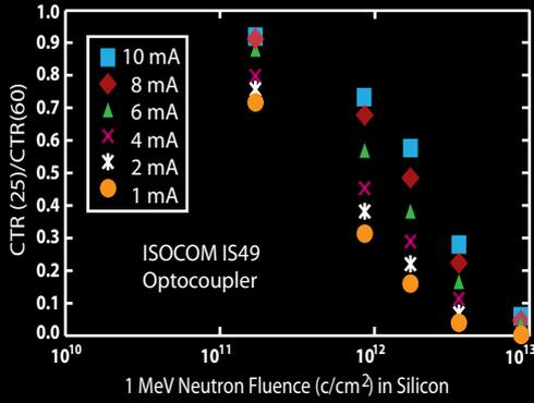
Fig. 1. Normalized CTR versus the radiation level for the IS49.
