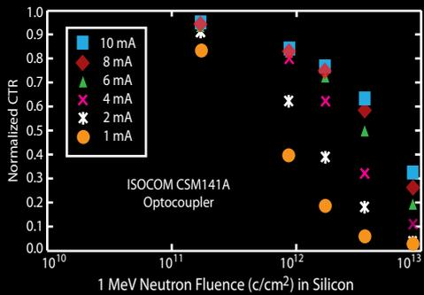
Fig. 5. Normalized CTR versus the radiation level for the CSM141A.
