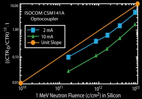
Fig. 6. Values of  $[(CTR_0/CTR)^{1/3} - 1]$  for  $I_F = 2$  and 10 mA for CSM141A.
