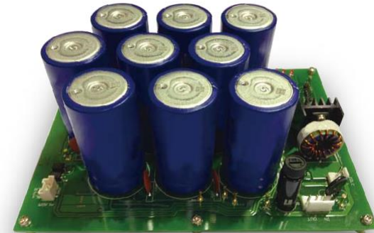
Capacitor UPS-J (PCB-type)
