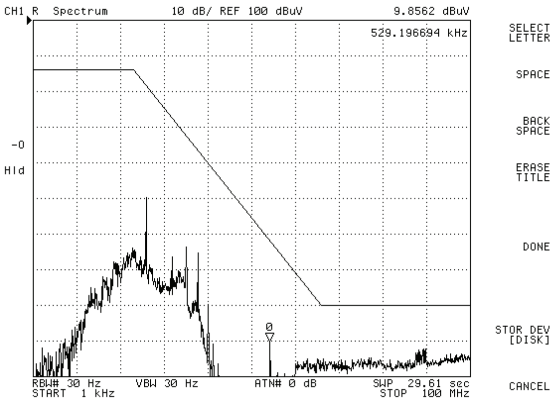
Fig 2. Positive Input Line with SF461 GEN II EMI Filter for V_{IN} = 28V and Rated Load, S2805S
