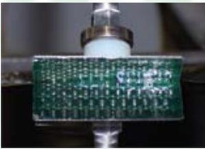
The worldwide conversion to lead free (Pb-free) electronics has resulted in a change to the solder ball alloy used on BGA packages from tin-lead (SnPb) to
